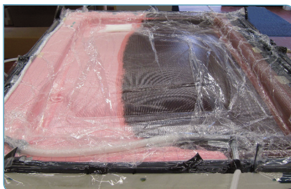
The new Fibretemp process produces large carbon fibre parts without the use of an oven or autoclave
