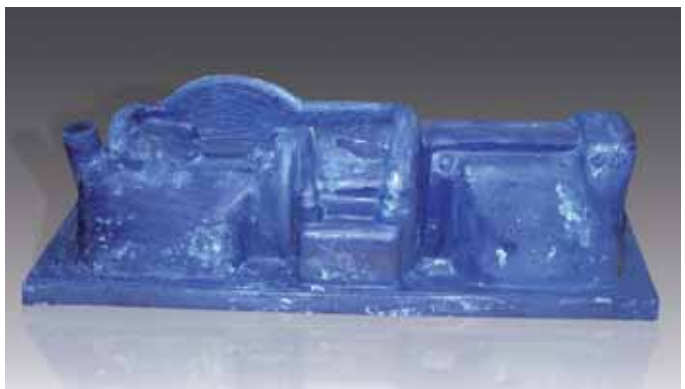
Blank for electroplating bath model dashboard of ebablock ® W mineral blue Picture credits: Heinz Gaubatz Modell- und Formenbau GmbH / Galvanoform GmbH
