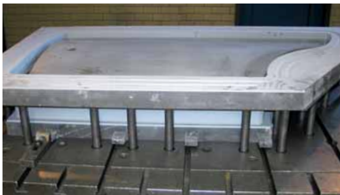
Sheet metal forming tool of ebablock ® W (outside door layer of a luxury sedan)
