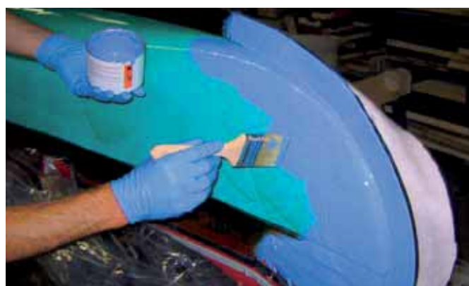
Application of the surface layer
