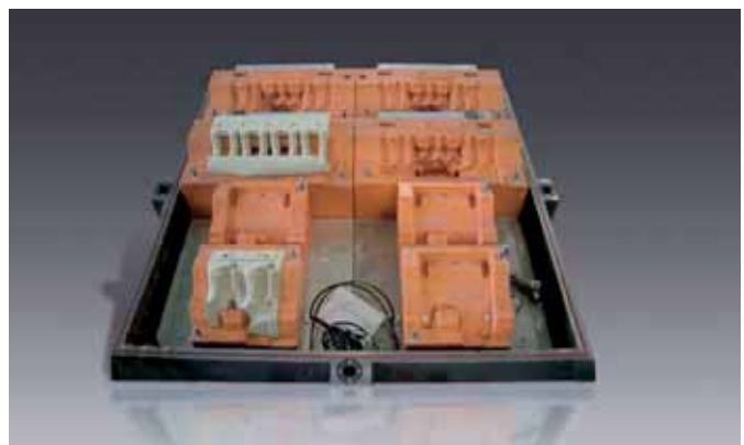
8-fold core box made of ebablock® K with core nests
