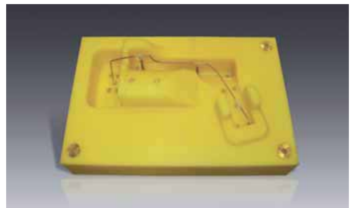
Core box made of ebablock® M 04
