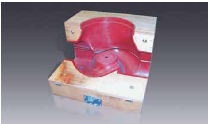
Core box made of OH 11 with PS 03
